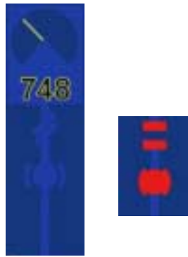
Figure 6. Propulsion and gear/brake-system, to the right the gear is not connected while the brake is engaged.
