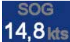
Figure 4. Speed over ground, presented in digits with an accuracy of one decimal.
