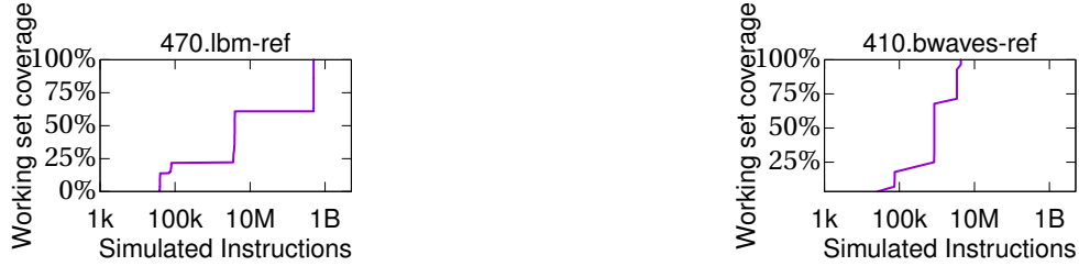
Fig. 1: The coverage of the working set as a function of the simulated interval. Warming the complete working set of 470.lbm (required for a large DRAM cache) requires almost 1 B instructions.
