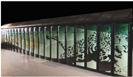
Cray XT Jaguar, 181504 Opteron cores, 362 TB main memory, 1,65 Pflap peak performance (Nov 10 2008). Located at ORNL, USA
