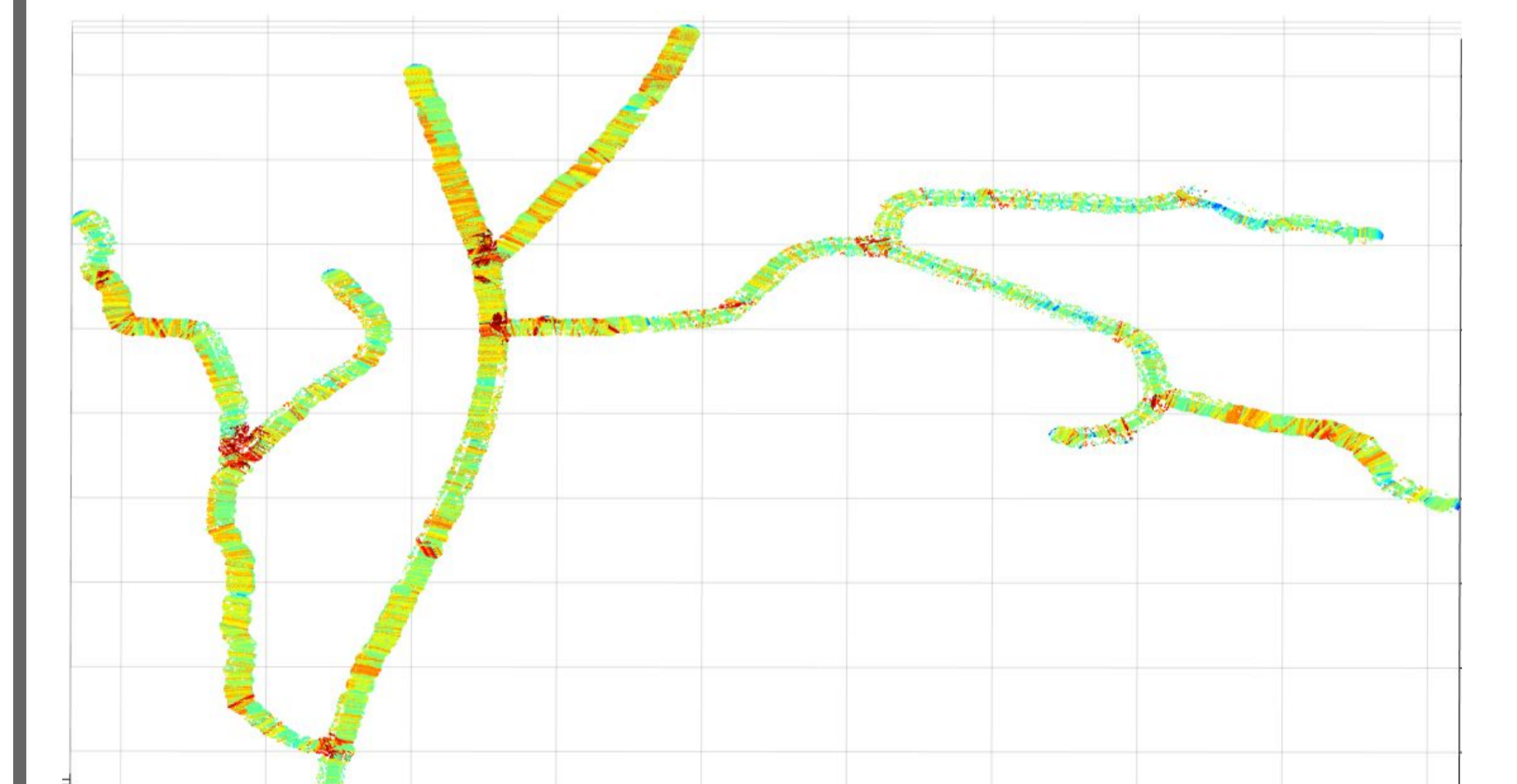
The road width. The colors represent the width in meters. However the width is actually the width of the whole flat surface, not only the road.
