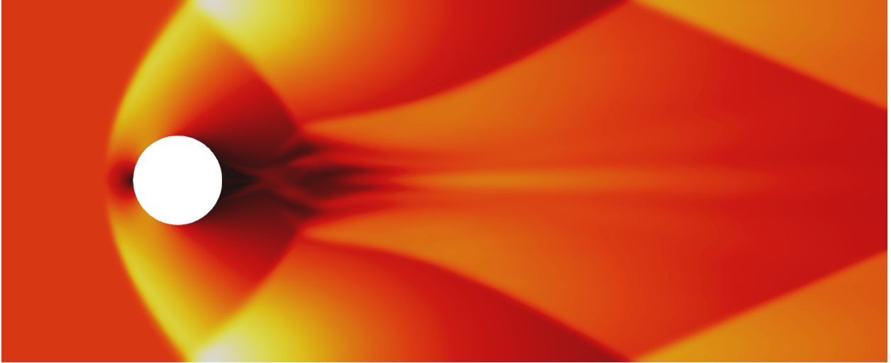
Figure 9: The numerically computed B-field at time T=0.5 for the Cylinder problem with 35313 \mathbb{P}^1 nodes using the projection method.
