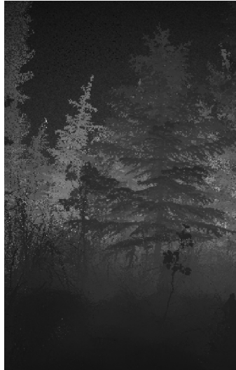
Figure 13: Laser image showing the distance to the objects in the direction away from the laser.
